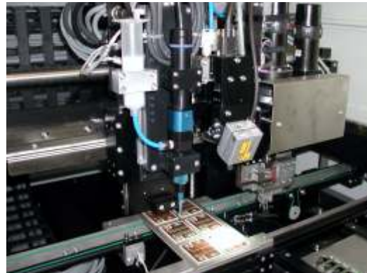
In-Line Multifunctional XCEL for dispensing and assembly on DCB substrates for power modules
